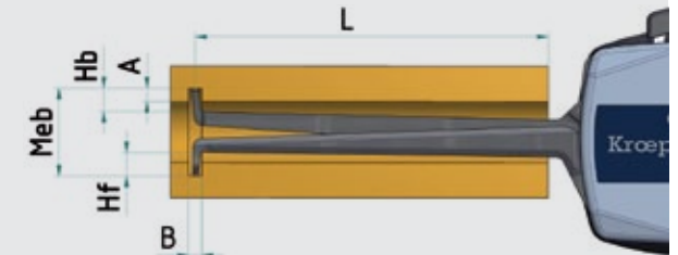
Meb Measuring range A Groove depth B Groove width Hb Measuring contact movable Hf Measuring contact fixed L Measuring depth
