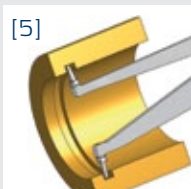
[5] Ball Ø 1,0 mm Ball Ø 2,0 mm
